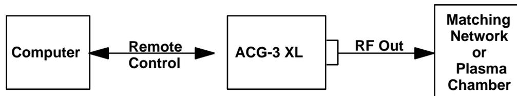
The remote control connection allows a computer or external control unit to adjust and read back power via the accessories connector (See Section 3.3). The RF out connection is made to either a load (often a plasma chamber) or a matching network.
